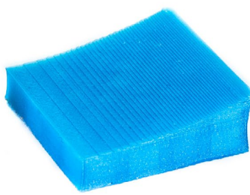
How the layer height affects the object's surface
